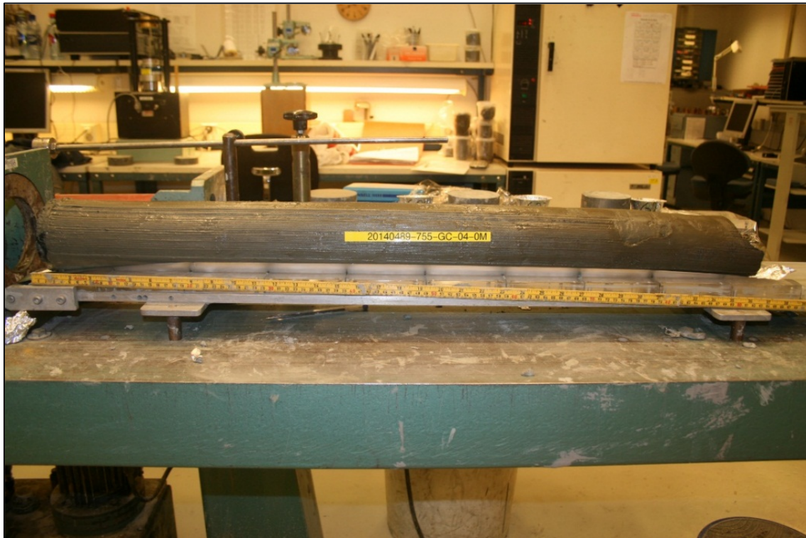
Figure 30 Gravity corer sample 755-GC-04 at the laboratory.
