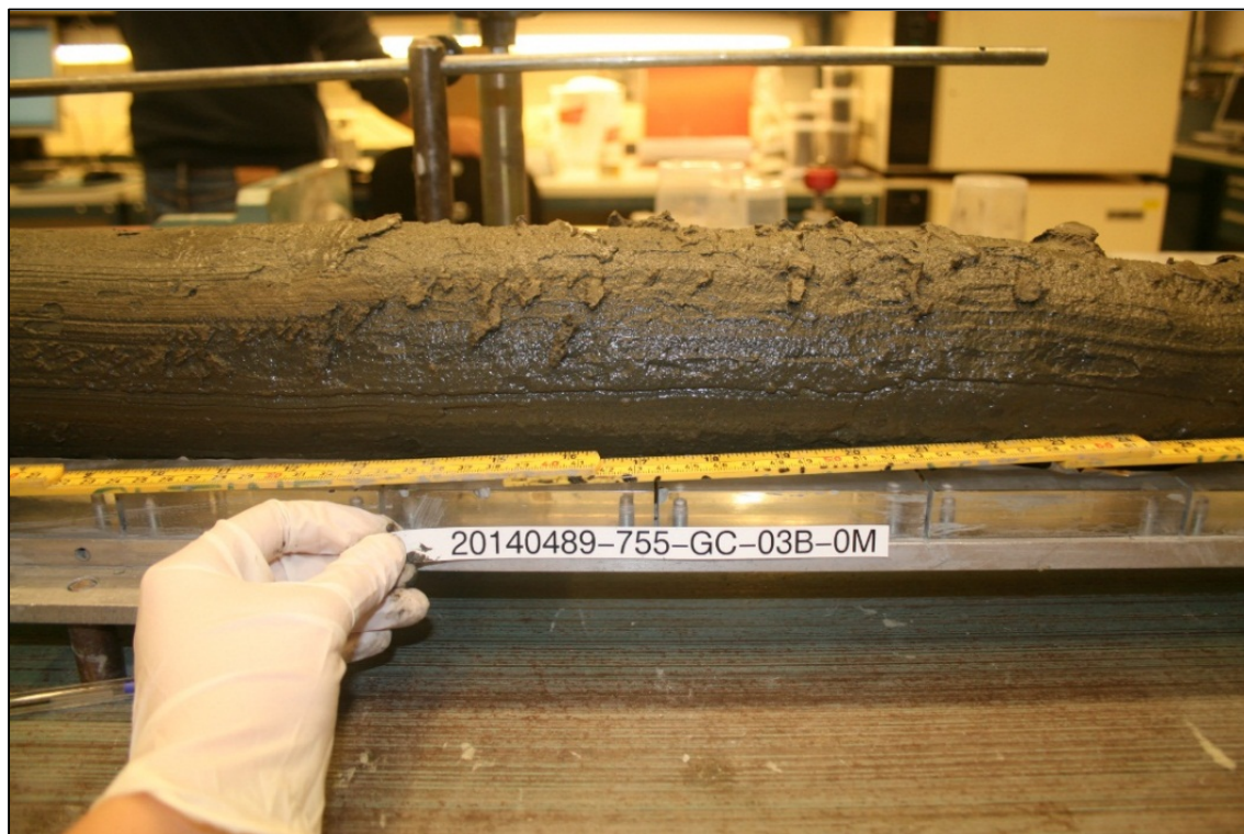
Figure 29 Gravity corer sample 755-GC-03 at the laboratory.
