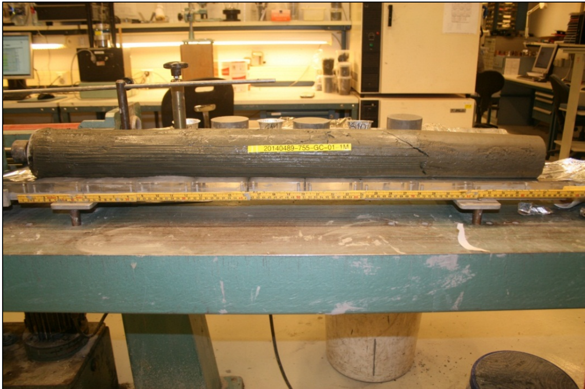
Figure 27 Gravity corer sample 755-GC-01 at the laboratory.
