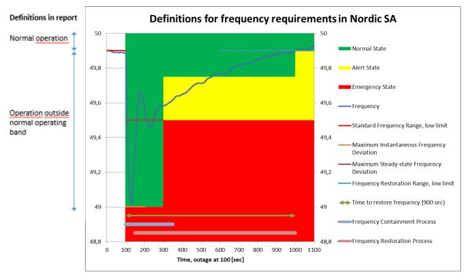
Figure 6 Definitions for frequency quality criteria, based on definitions in Article 42 in [8] and Article 8 in [26].
