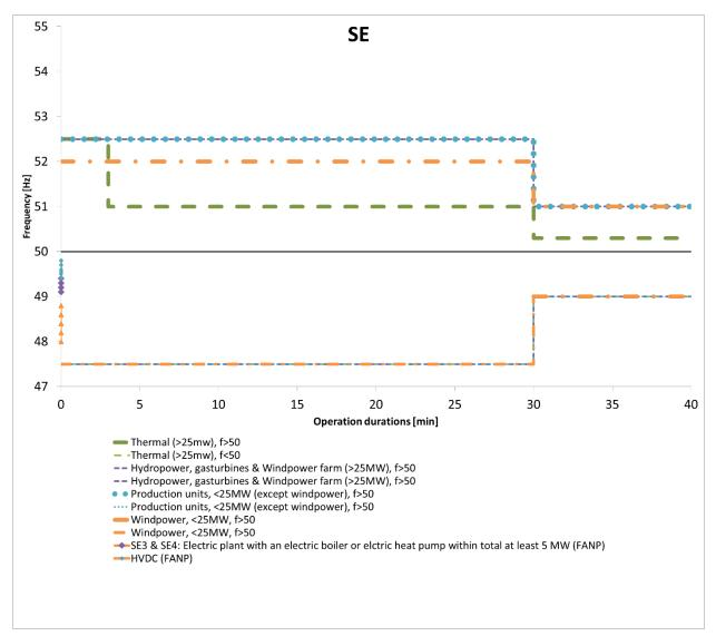
Figure 39 Frequency minimum levels, time scale 0-40 minutes, Sweden.
