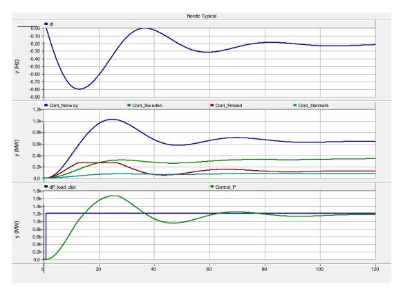
Figure 32 Responses in case of 1200 MW loss of production. From top: Frequency deviation / Reserve power responses of each TSO / Power trip and total control power response. Inertia 10000MWs/Hz, FBF = 5230 MW/Hz, Control with present time constants according RAR report. See footnote 23.
