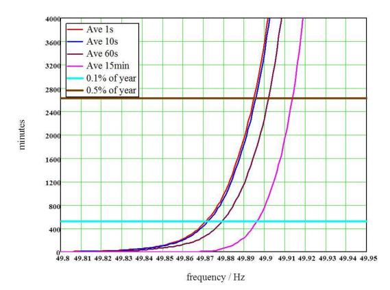
Figure 11 Minutes below the SFR during the year 2008 in Nordic grid measured with different sliding averages.
