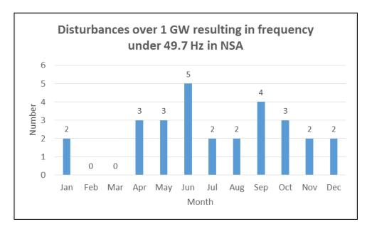
Figure 27 Monthly distribution of frequency drops deeper than 49.7 Hz in years 2003-2013.
