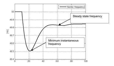
Figure 7 Simulated frequency development when a disturbance occurs. Simulation model from [36] used.
