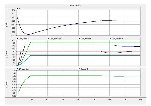
The hard limiters limits the control power to obliged power of each TSO.
