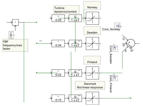
Figure 29 Simulation model used for illustration. The FBF is shared for each TSO in same proportions as reserve obligations. Time constants are according to above table from RAR report [36]. See footnote 23.
