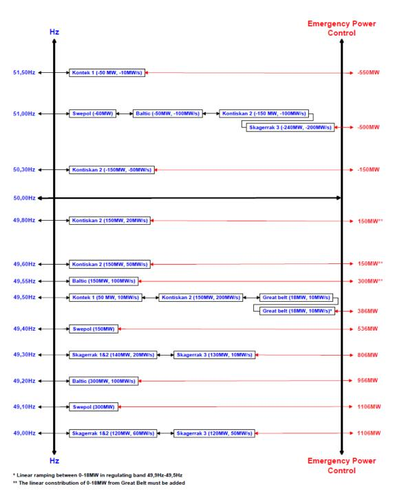
Figure 8 HVDC emergency support in the NSA.
