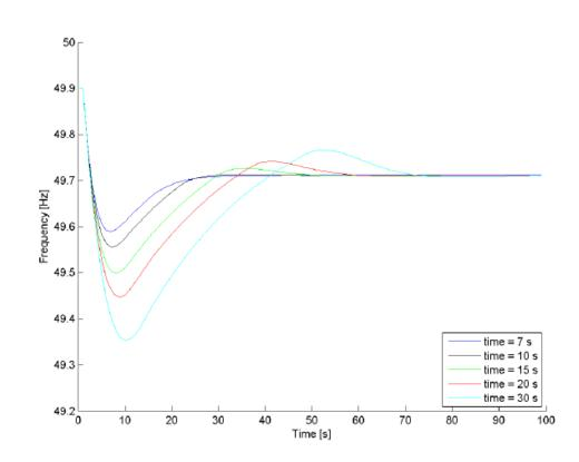
Figure 25 Relations between speed of FCR and frequency network characteristic for steady state frequency deviation of 49.7 Hz (frequency deviation after outage is 200 mHz). Loss of production is 1300 MW, FBF 6500 MW/Hz, Inertia 250 GWs [38].
