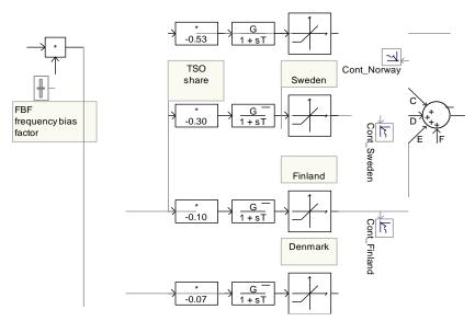
Figure 31 Simulation model used for illustration. The FBF is shared for each TSO in same proportions as amount of reserves. Time constants are according to above table from RAR report. The limiters are not active. See footnote 23.
