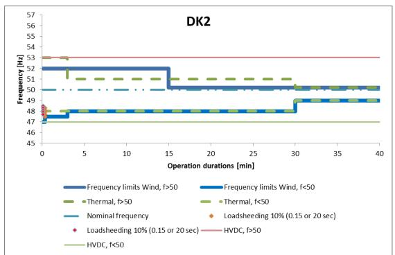
Figure 38 Frequency minimum levels, time scale 0-40 minutes, Denmark (DK2).
