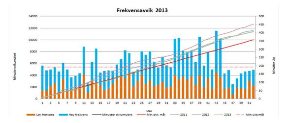
Figure 3 Frequency quality in 2013 – total minutes cumulative on the left and weekly bar on the right [from Statnett weekly report on frequency quality]
