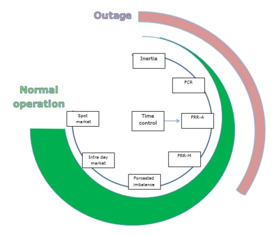
Figure 12 Relations of activated power between Load-Frequency Control elements. The figure indicates, in principle, the relative size of power from spot market to inertia. It should be noted that the activation order for normal operation and operation outside normal operating band is the same, and moves from inertia to FRR-M. I.e. the "time-line" does not continue from FRR-M to spot market, but arrow is continued to show the relative sizes of power.
