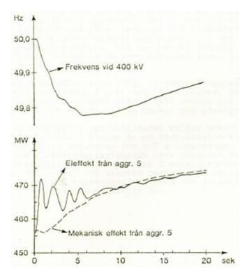
*Figure 16 The difference between mechanical and electrical power during a frequency disturbance.* [24]
