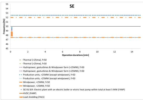
Figure 40 Frequency minimum levels, time scale 0-14 minutes, Sweden.
