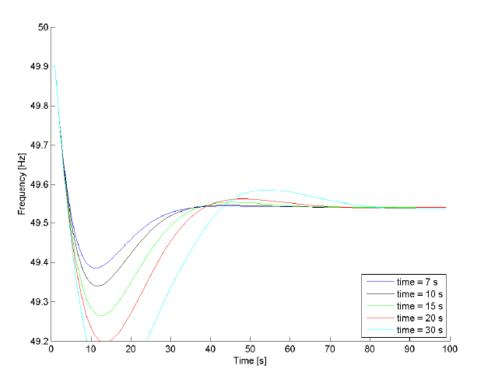
Figure 24 Relations between speed of FCR and frequency network characteristic for steady state frequency of 49.5 Hz (frequency deviation after outage is 400 mHz). Loss of production is 1300 MW, FBF 3250 MW/Hz, Inertia 250 GWs [36].
