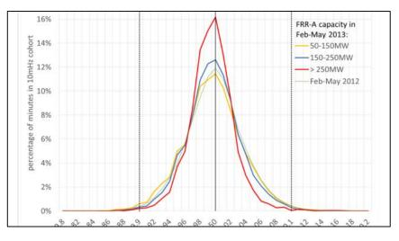
Figure 5 Distribution of frequency, separate for three levels of FRR-A during the test period from February to March 2013. [42]
