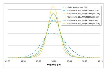
Figure 20 Different setting and requirement for the response of FRR-A will all fulfil the need - keep the frequency within the Standard Frequency Range [36].
