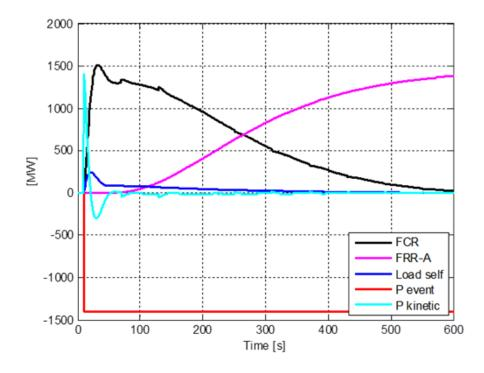
Figure 10 An illustration of calculated power contributions after tripping 1400 MW production. Note: only illustrative figure (not measured response from real disturbance). RAR-model used for simulation [36].
