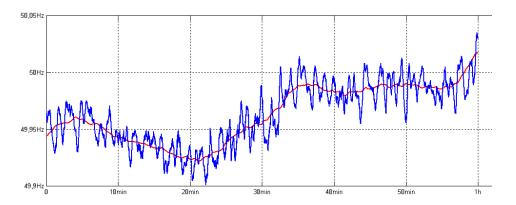
Figure 18 Original frequency measurement (blue) and a filtered frequency (eliminating the 60 s oscillation) (red) [41]
