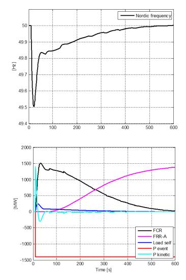
Figure 14 Response of Inertia, FCR and FRR-A after an outage.
