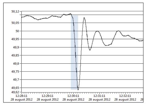
Figure 22 Frequency during a loss of larger production unit in the Nordic synchronous system. Area of inertial response highlighted.
