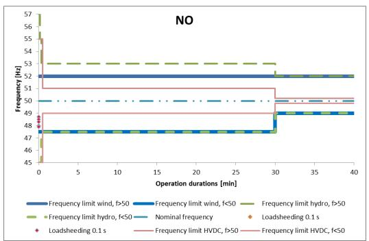
Figure 35 Frequency minimum levels, time scale 0-40 minutes, Norway.
