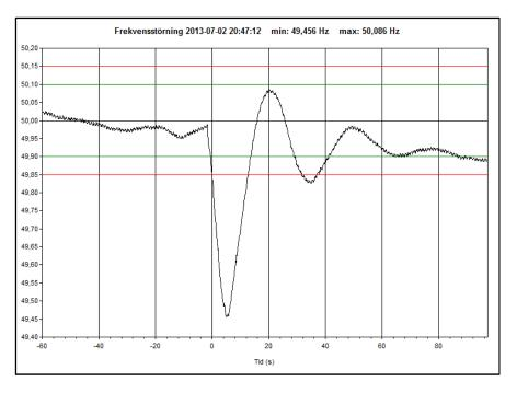
Figure 4 Typical frequency profile after forced outage of a large production unit (nuclear power plant).
