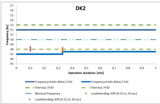
Figure 37 Frequency minimum levels, time scale 0-1 minutes, Denmark (DK2).
