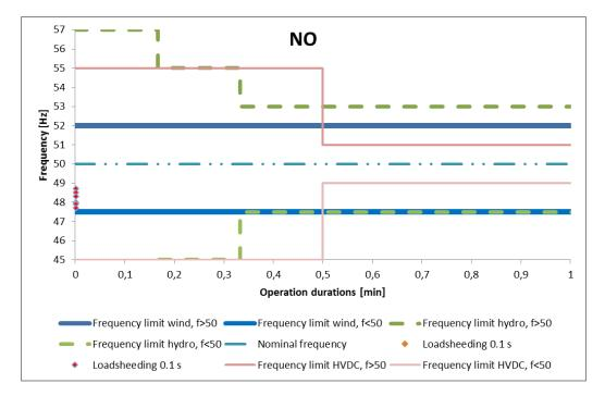
Figure 34 Frequency minimum levels, time scale 0-1 minutes, Norway.
