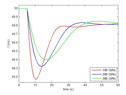
Figure 23 Simulated response for frequency response when losing a large generating unit, as a function of different system inertia levels.
