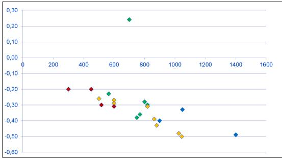
Figure 28 Frequency drop (Y-axis) vs tripped power (X-axis) in disturbances 2009-2012. Inertia: < 150 GWs, 150-200 GWs, 200-250 GWs, 250 -300 GWs
