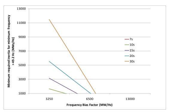
For a low value of inertia (50 GWs)<sup>17</sup> and a low value of FBF (3250 MW/Hz), the FCR response needs to be 10 sec or faster to prevent the frequency from going below 49.2 Hz.
