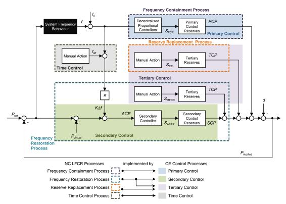
*Figure 13 The control loop of the Load-Frequency Control (from Drafting team Policy 1 ENTSO-E CE)*
