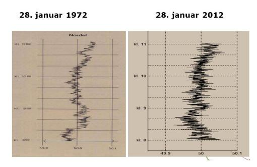
Figure 2 Oscillations have increased in 40 years ([35] and 2012 measurement values from ENDK Scada system)
