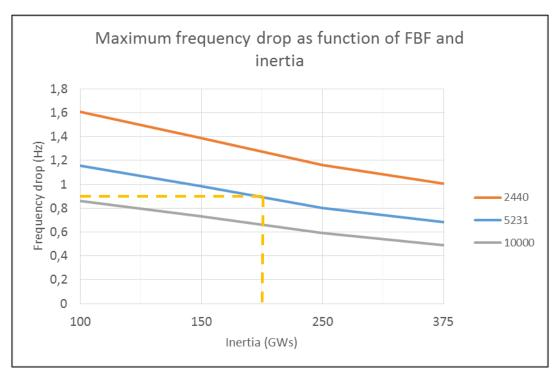
Figure 33 Maximum instantaneous frequency drop (y-axis) vs. inertia (x-axis) and FBF (orange, blue, grey) as parameter. Yellow dashed line represents value in summary of analyses, section 9.4.
