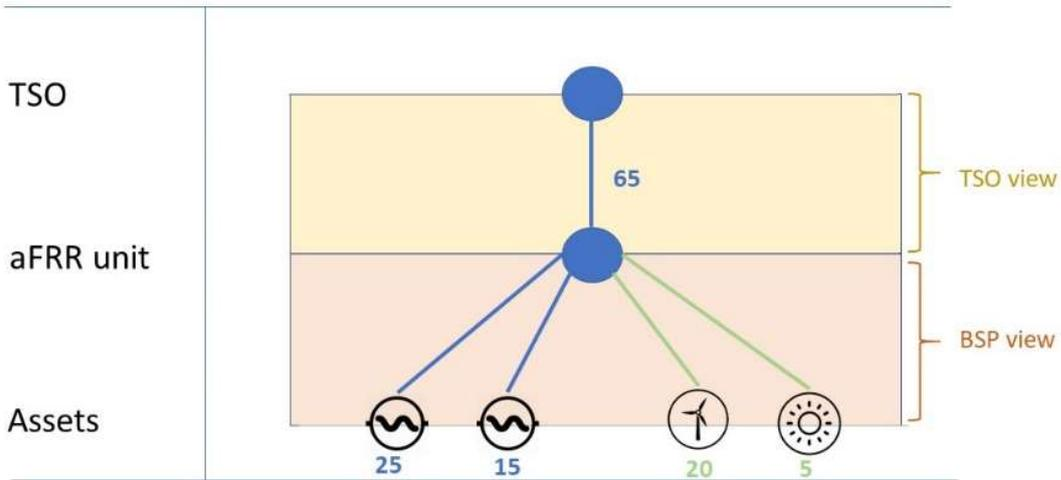
Figure 1: The diagram illustrates the communication flow between the TSO, aFRR unit and the power producing assets
