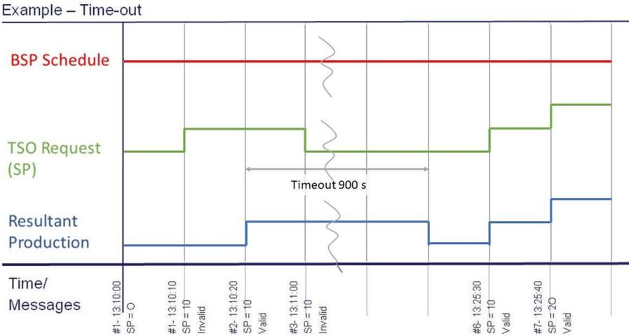
Figure 4: Description of the timeout functionality. The resultant production does not change in the timeout period.
