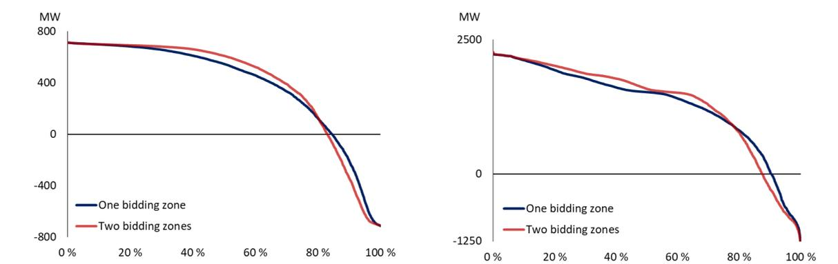
Figure 2: Simulated power flow on the line between NO4 and SE1 (left) and total flow out of NO4 (right), with one or two bidding zones. The capacity between NO4 and SE1 is limiting in many hours, and with NO4 split, the model is capable of increasing flow on the line/lines slightly in hours where they are already highly loaded. The result is from a simulation of 2025, and we use Flow Based Market Coupling (FBMC).
