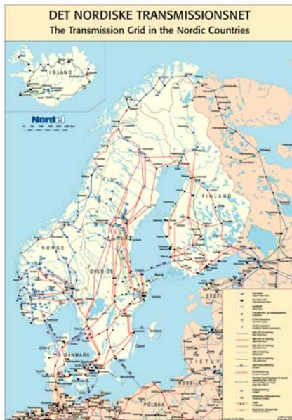
Fig. 1. The Nordic transmission grid
